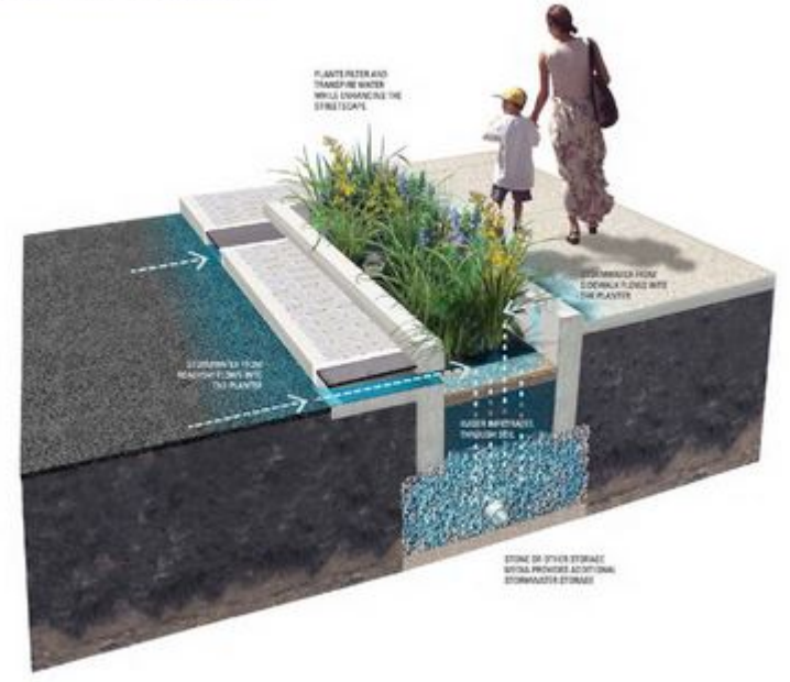
Figure 2.1: Three-Dimensional View of a Stormwater Planter
